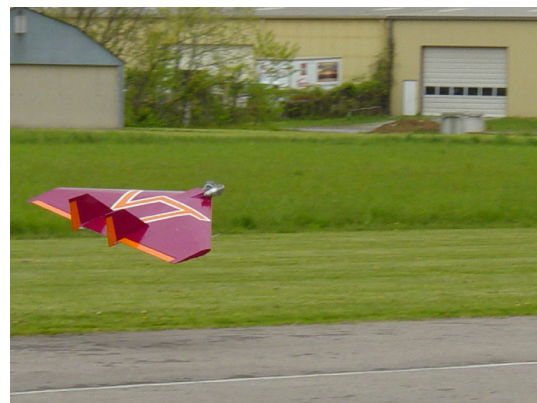
Figure 4. A takeoff of the delta vortex (note pitot tube on onboard wing station)
