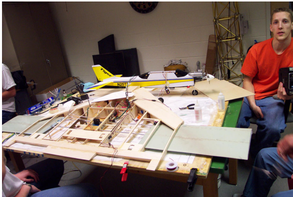
Figure 5. The morphing wing under construction at Virginia Tech
