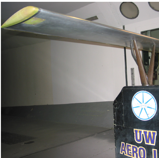
Figure 2. Wing Mounted in Test Section
