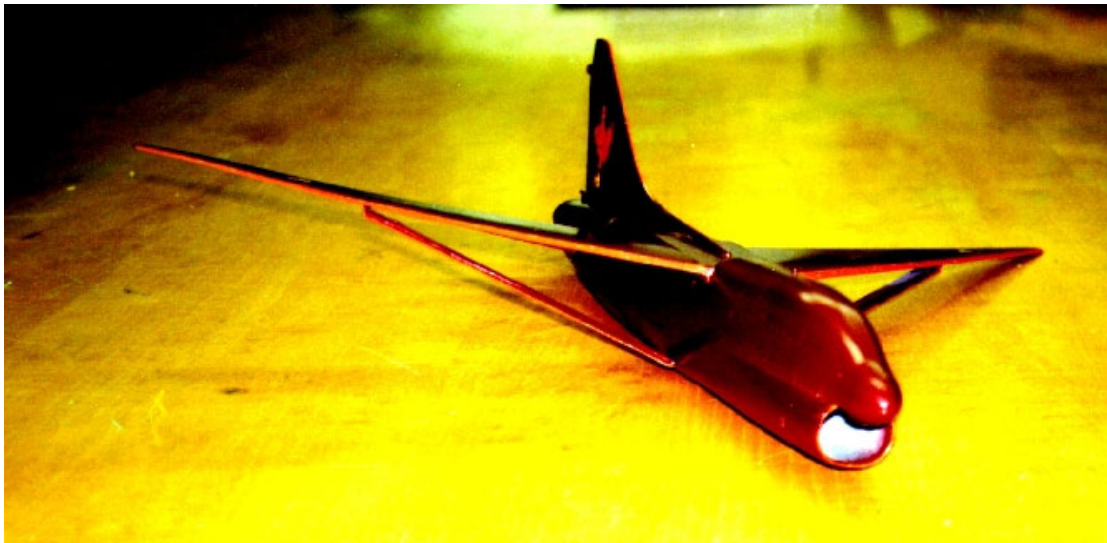
Figure 3: Picture of the A7 SBW demonstrator aircraft made by the senior class design team ( Team RevCon).
