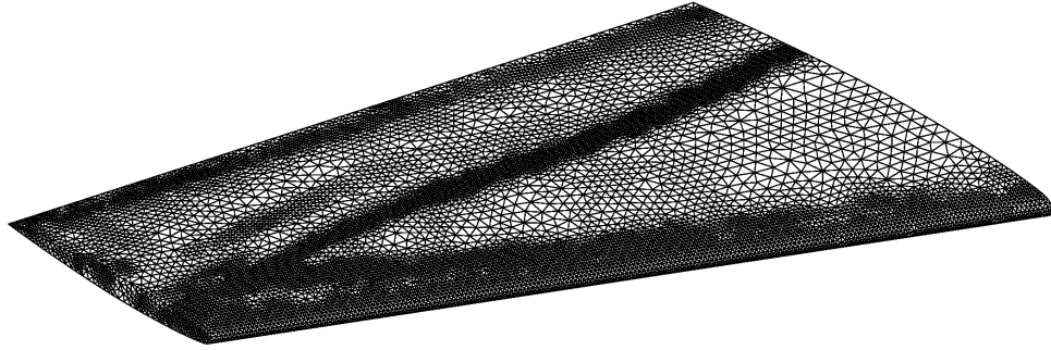
Figure 16: Surface triangulation of the ONERA M6 wing (re-meshed case)
