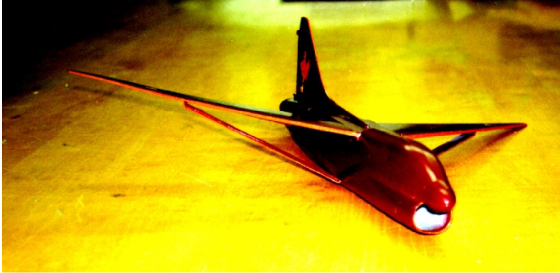
Figure 1-1. The strut-braced wing concept as it might be demonstrated on an A-7.
