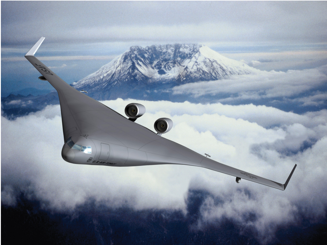
Figure 1: A blended-wing-body aircraft with a conventional propulsion arrangement.
