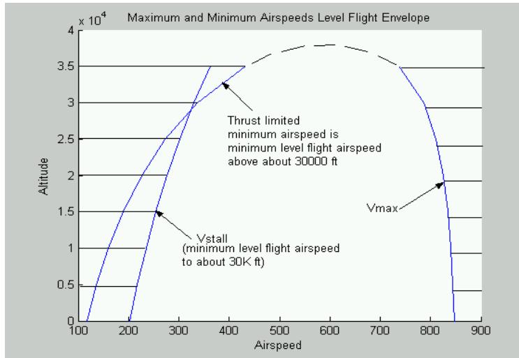
Here the hatched area indicates the area outside of the flight envelope of this aircraft.
