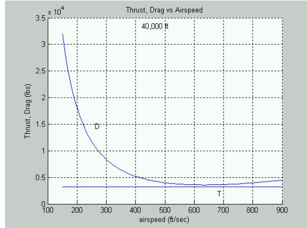
Here we see that the thrust at 40,000 ft is not sufficient to equal the drag at any speed and hence there is no solution. Consequently, the “ceiling” of the aircraft is less than 40,000 ft. The tables that accompany these graphs and the one at sea level follow:
