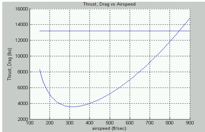
simple (constant thrust and constant drag parameters  $C_{D_a}$  and K, we can solve for the max and min speed directly:
