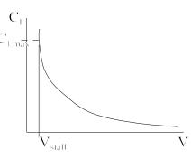
upper limit to the lift coefficient called  $C_{L_{max}}$ , and it occurs at the angle-of-attack called the stall angle-angle-of-attack,  $\alpha_{stall}$ . Furthermore, the speed at which this maximum lift coefficient (or  $\alpha_{stall}$ ) is called the stall speed,  $V_{stall}$ . (Many other important speeds, especially those required for take-off and landing, are based on the stall speed).
