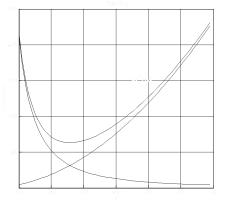
condition for maximum L/D. Note that the *max L/D does not occur at C\_{L\_{max}}* Furthermore, since  $L/D_{max} = C_L/C_D_{max}$  the value of maximum L/D is independent of altitude.
