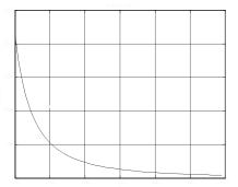
The second term is called the induced drag or drag-due-to-lift. It behaves in an unusual way as indicated in the figure. Here we note that the drag *decreases* as the airspeed increases. This behavior is counter intuitive! This portion of the total drag is the cost that we have to pay for using the air to hold up the aircraft. The faster we go, the easier it is for the air to hold up the vehicles since it has to deflect the air less to create the same lift (= weight).
