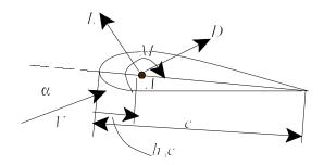
The drag is parallel to the relative wind, and the lift is perpendicular to the relative wind. The aerodynamic moment is positive nose up. Here we are taking the moment about point A. Once we pick a point, we can use some theorems from statics that say that we can represent and force and moment system by assuming that the forces act thorough a given point and that there is a pure moment about that point.
