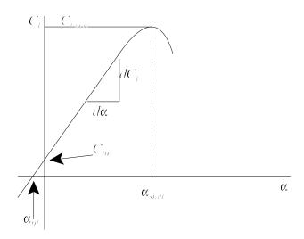
There are two intercepts that we can designate, one the alpha axis for zero lift, designated as  $\alpha_{0L}$ , the zero-lift angle-of-attack, and the one at zero angle-of-attack designated at  $C_{L_0}$ , the lift at zero angle-of-attack.
