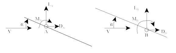
nce the wings are identical we can expect that the aerodynamic forces will be the same. The moments will not be the same since the *reference point is different*. From this observation we can state that:
