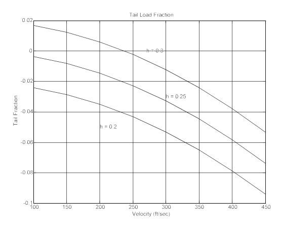
We can see for aft cg positions, the tail load can be positive, while for forward cg positions, the tail load is generally negative for all speeds.
