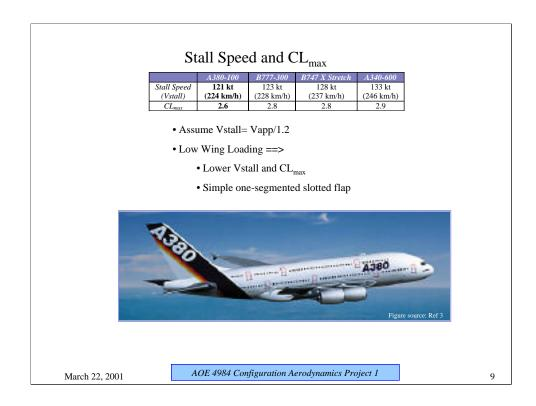
Due to large wing area and low wing loading, both stall speed and  ${\rm CL}_{\rm max}$  are lower than the other planes which have higher wing loading.
