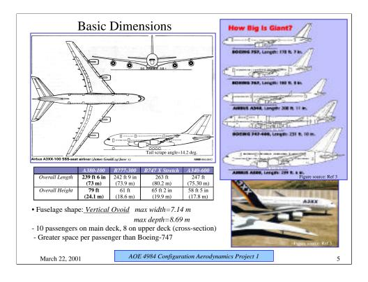
Tail scrape angle has been measured by using the layout figure of A380-100. Since the height of the landing gears is not specified, this approximation may not be accurate enough.
