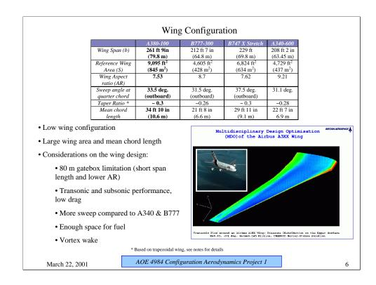
The taper ratio for each plane has been determined by using layout figures, and due to the measurement errors, the results may not be accurate.
