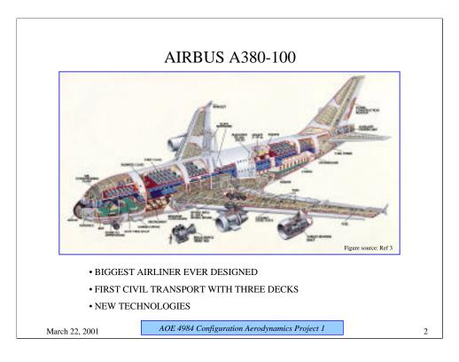
Airbus A380 is the biggest airliner ever designed. It will become the first full-triple decked large-body, long-range civil transport. Despite its large size, basic configuration of A380 is similar to a typical civil transport.
