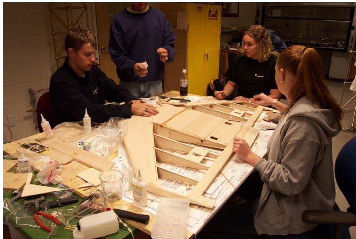
Figure 3.2: Delta Vortex under construction
