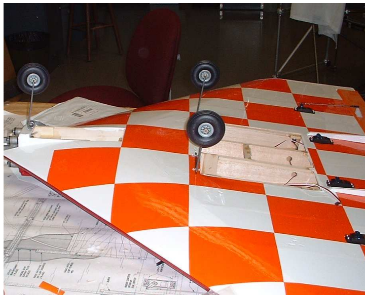
Figure 3.3: Lower surface of Delta Vortex with visible landing gear and instrumentation hatch
