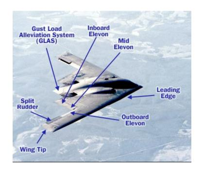
At low speed flight, drag rudders are open.
