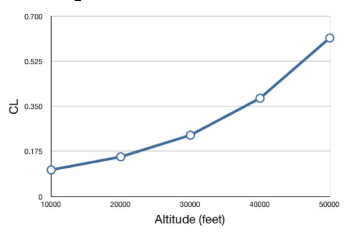
Data obtained from Lift equation at Mach = 0.79 and the corresponding densities for each altitude.
