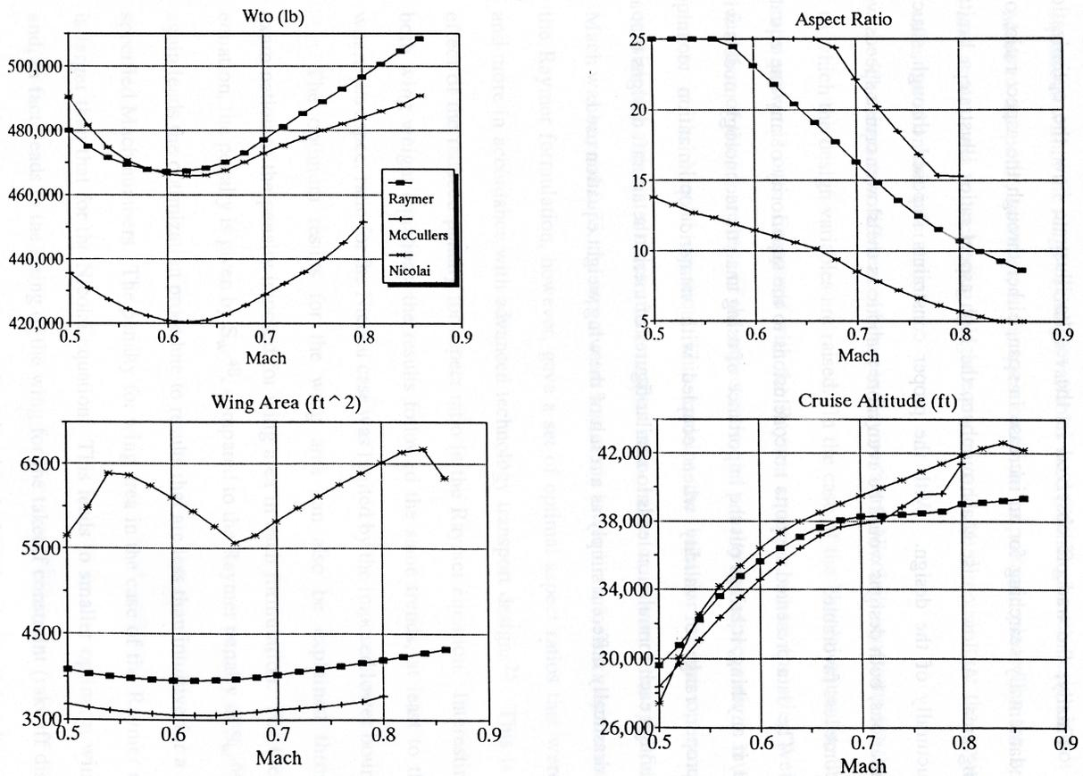
Figure 13. Effect of Increased Complexity (Wing Weight Models) on Optimum.
