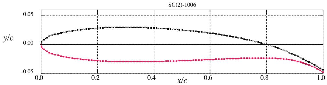
Figure C23-1. Whitcomb SC(2)-1006 airfoil (from NASA TP 2969). Not to scale.
