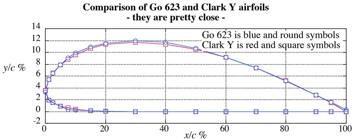
Figure C23-1. Comparison of Go 623 and Clark Y airfoils (not to scale).
