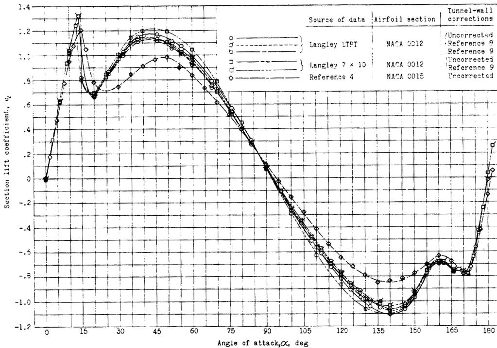
Figure 2. The 0012 over the full alpha range (NACA TN 3361.)
