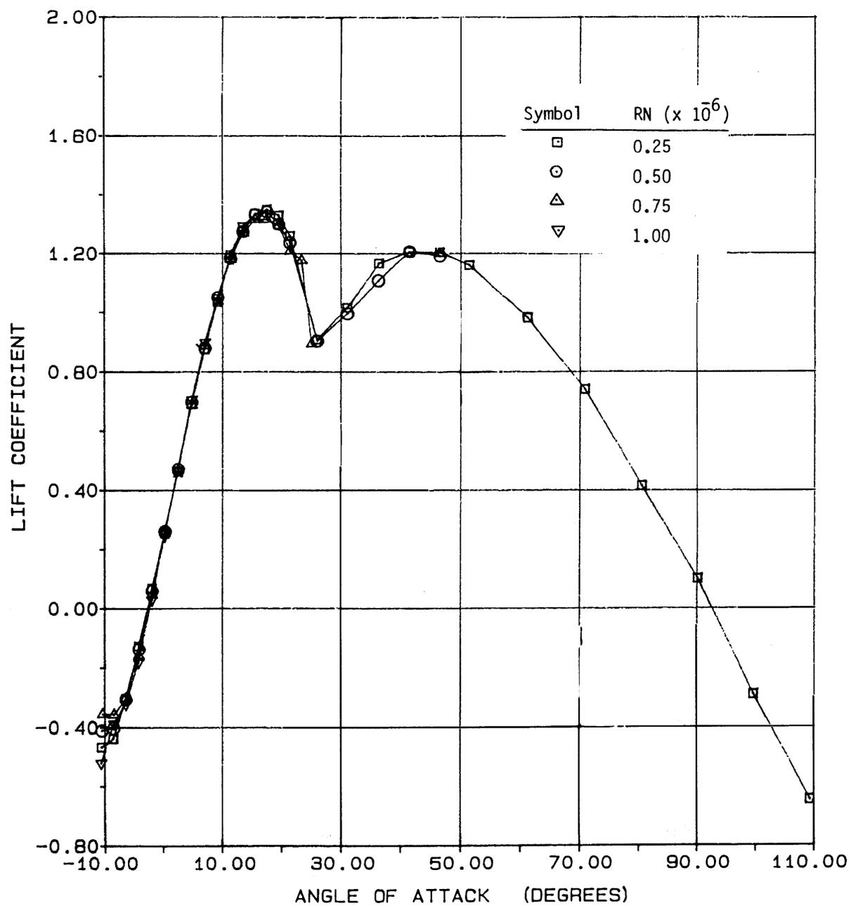
Figure 3. NACA 4412 lift for a "2D" case. (DOE data)
