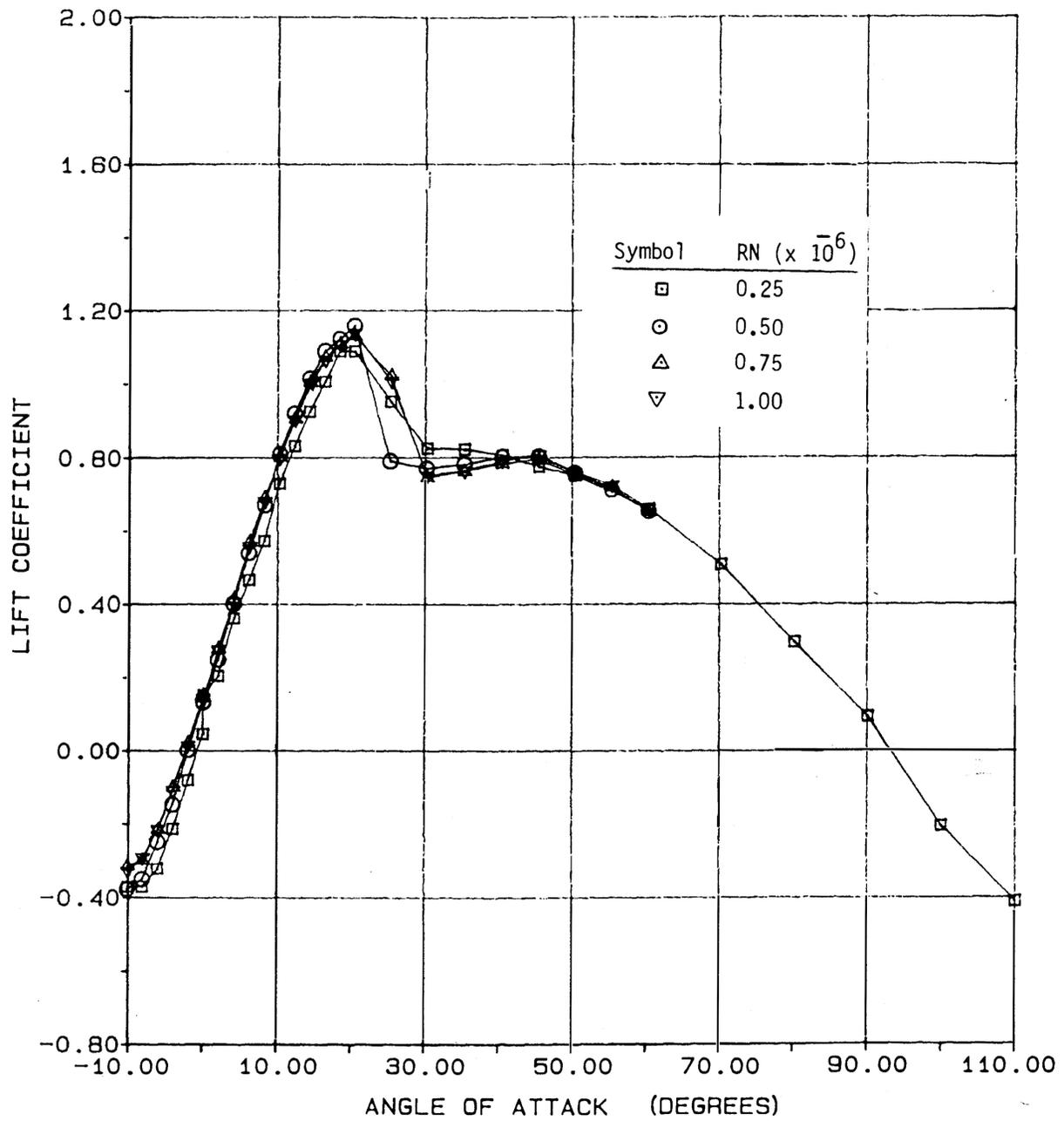
Figure 4. NACA 4412 lift for an AR = 6 case. (DOE Data)
