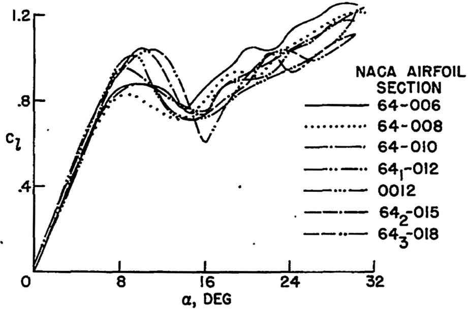
Figure 1. Loftin's collection of airfoil data (NACA TN 3241)
