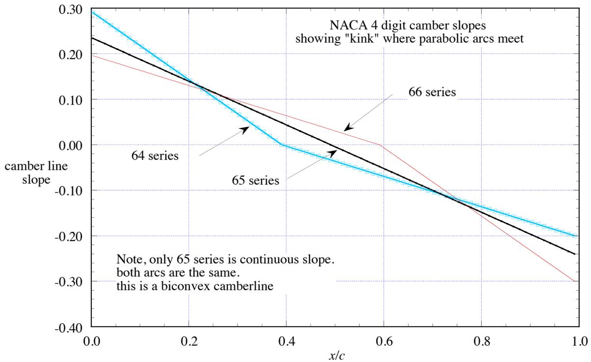
Figure 10. Comparison of camber line slopes for the NACA 4-digit series camberlines 64, 65, 66.
