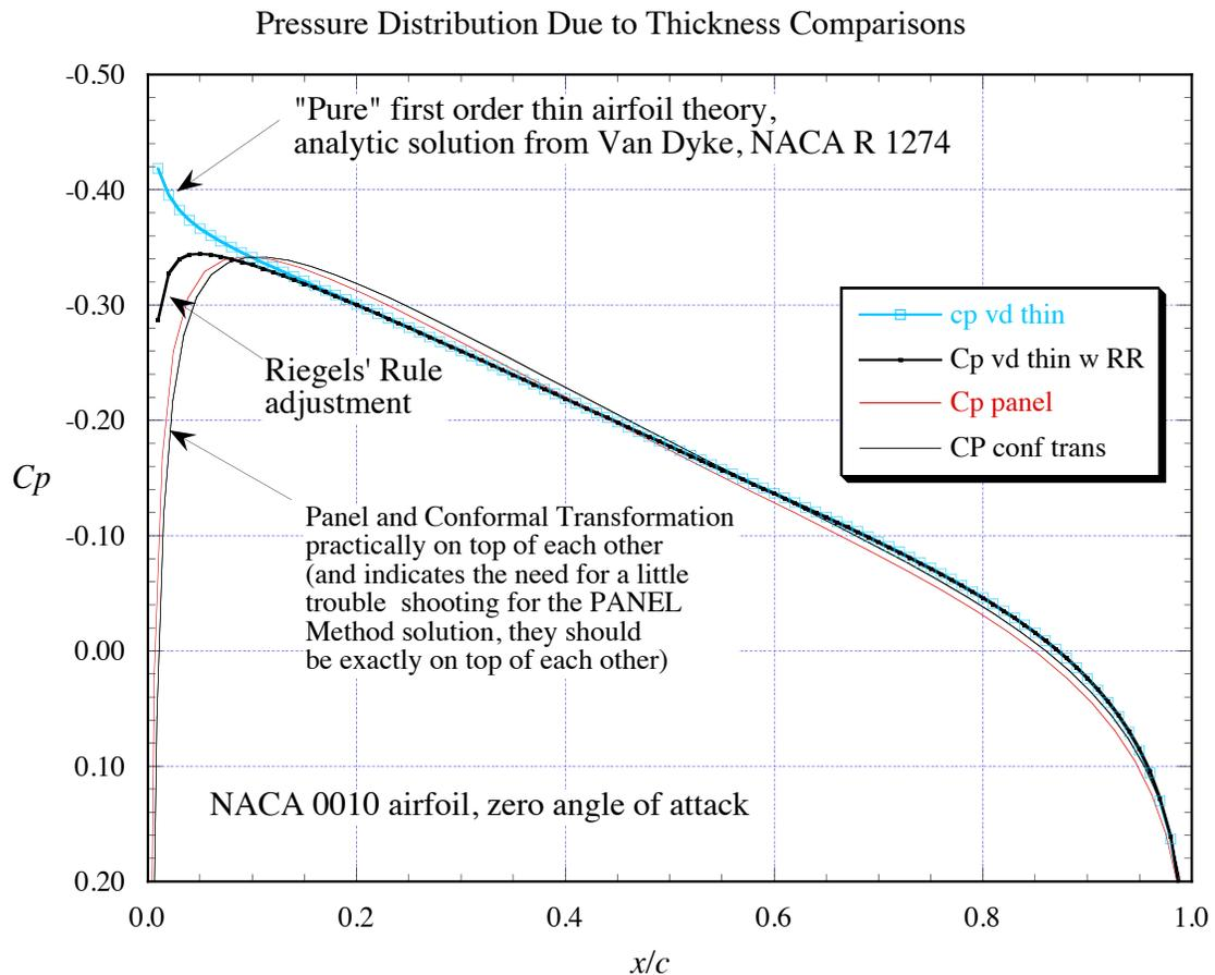
Figure 3. Comparison of pressures due to the basic thickness of the airfoil. Thin Airfoil theory compared to “exact” PANEL and Conformal Transformation methods. NACA 0010 airfoil at zero alpha.
