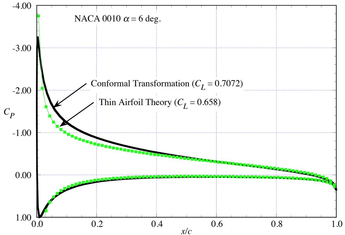
Fig. 8. Comparison of the pressure distributions for thin airfoil theory with conformal transformation results for an uncambered NACA 0010 airfoil at 6 deg. angle of attack.
