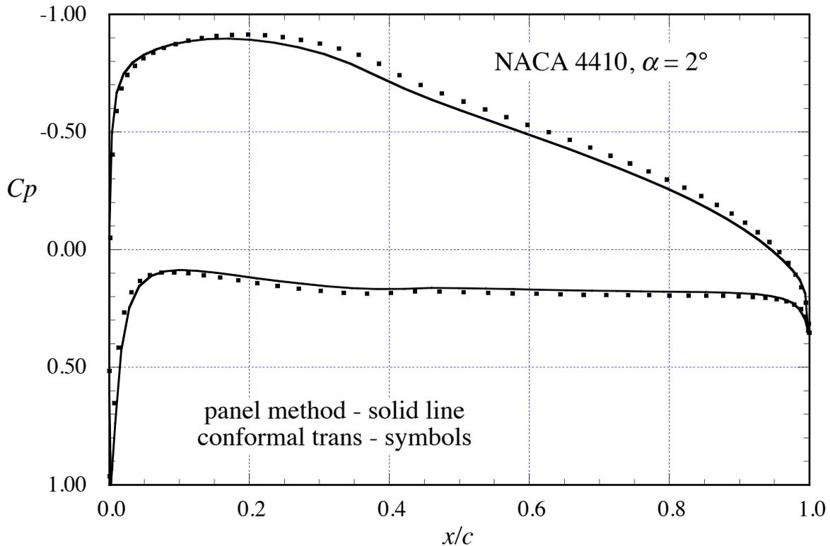
Figure 6. Panel and conformal transformation method results for the NACA 4410 airfoil at  $2^\circ$  alpha. The differences in the pressures appears pretty small.
