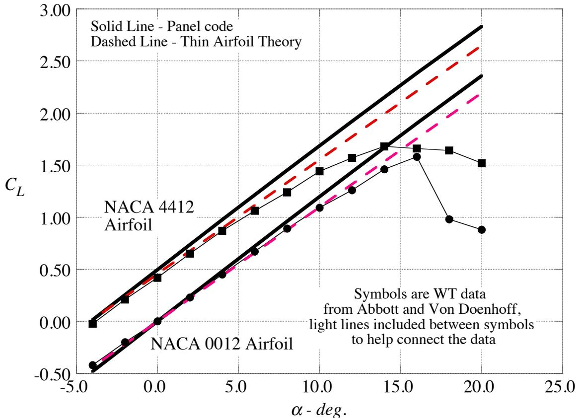
Figure 5. Comparison of the thin airfoil and exact panel method results for cambered and uncambered NACA 4-digit airfoils. Wind tunnel results are also included.
