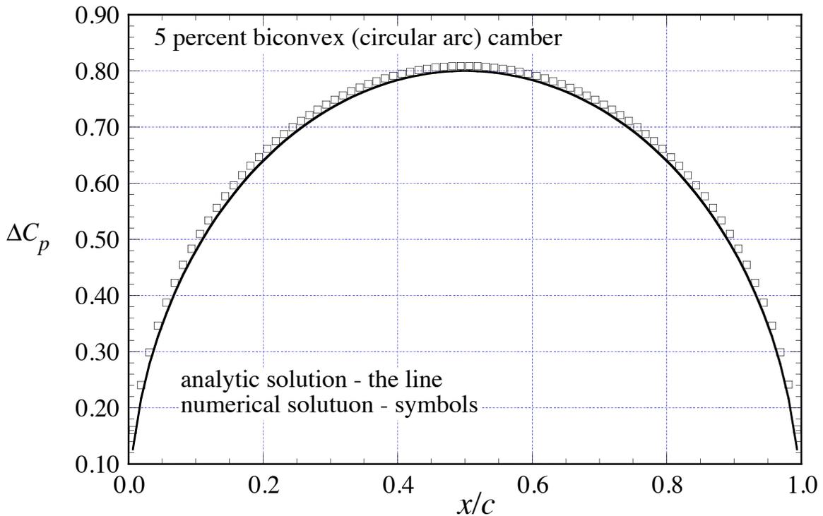
Figure 9. Comparison of analytic and numeric values of  $\Delta C_p$  for a 5% max camber biconvex camber line (also shown in Katz and Plotkin)
