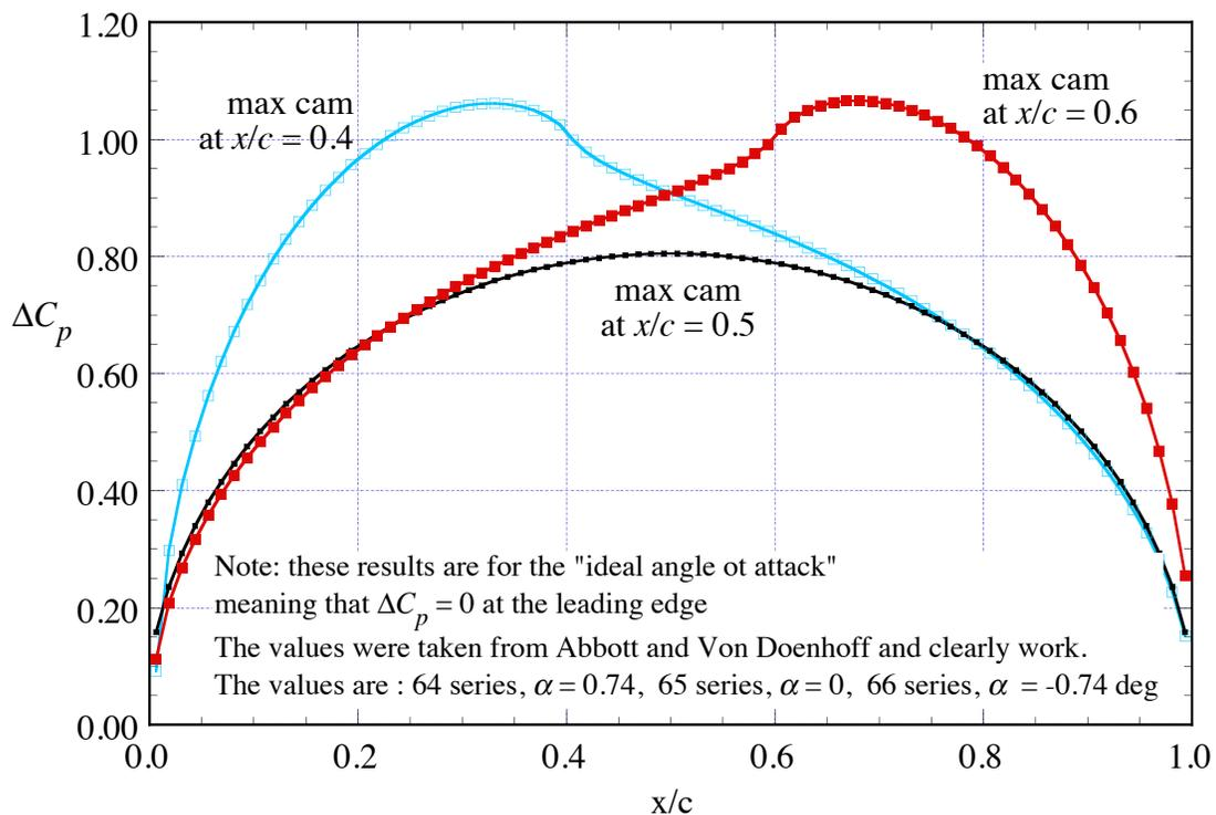
Figure 11. Chordloads for the NACA 4-digit airfoil camber lines at the ideal angle of attack.
