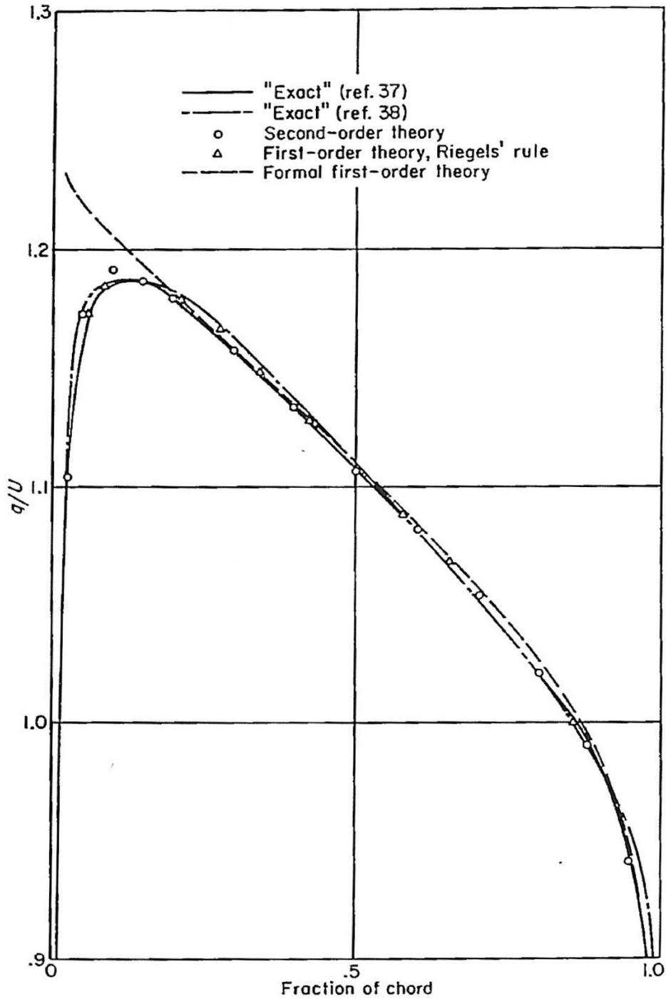
Figure 2. From Van Dyke (NACA R 1274). Comparison of surface speed predictions for an NACA 0012 airfoil at zero angle of attack.
