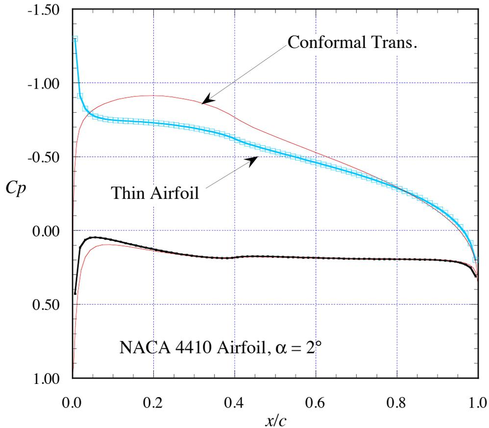
Figure 7. Comparison of the conformal transformation method and thin airfoil theory predictions for the pressure distribution on an NACA 4410 airfoil at  $\alpha = 2^\circ$ .
