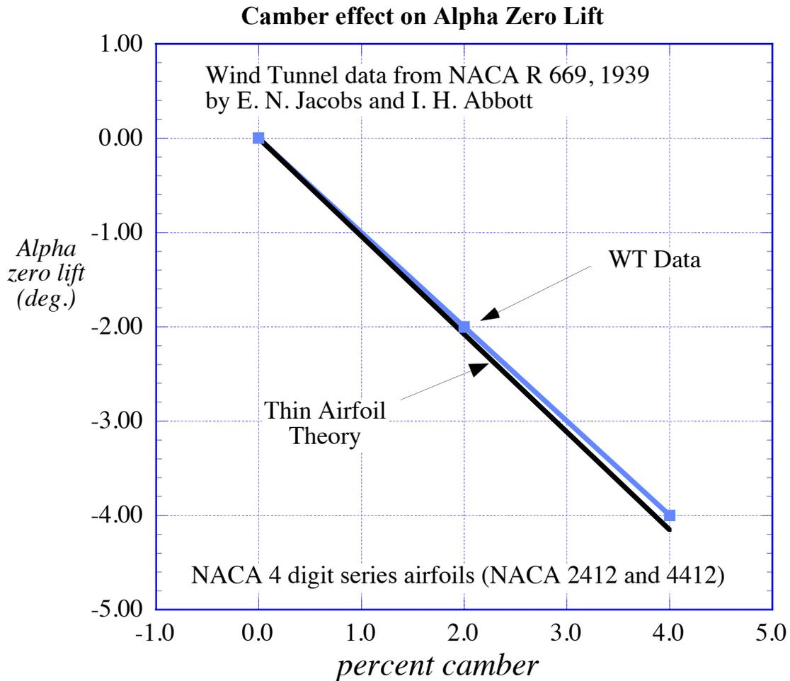
Figure 4. Comparison of the thin airfoil theory predicted zero lift angle of attack with wind tunnel tests for the NACA 4-digit camber lines at various values of the maximum camber.
