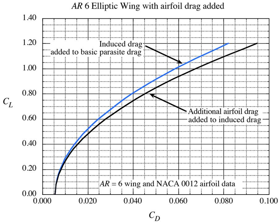
Figure 2. The  $AR = 6$  wing drag polar with the NACA 0012 airfoil drag from Abbott and Von Doenhoff added.
