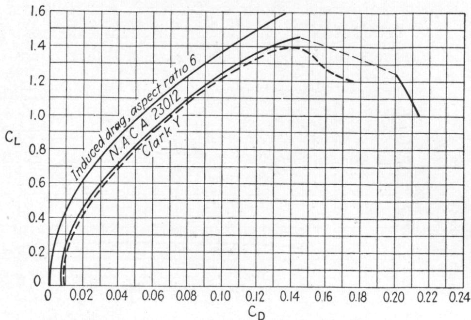
Figure 4. Warner's airfoil and induced drag polar (Fig. 96, pg 166)
