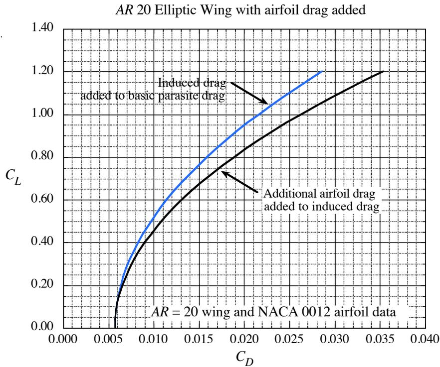
Figure 3. The  $AR = 20$  wing drag polar with the NACA 0012 airfoil drag from Abbott and Von Doenhoff added. Note difference in  $C_D$  scale compared to Fig. 2.
