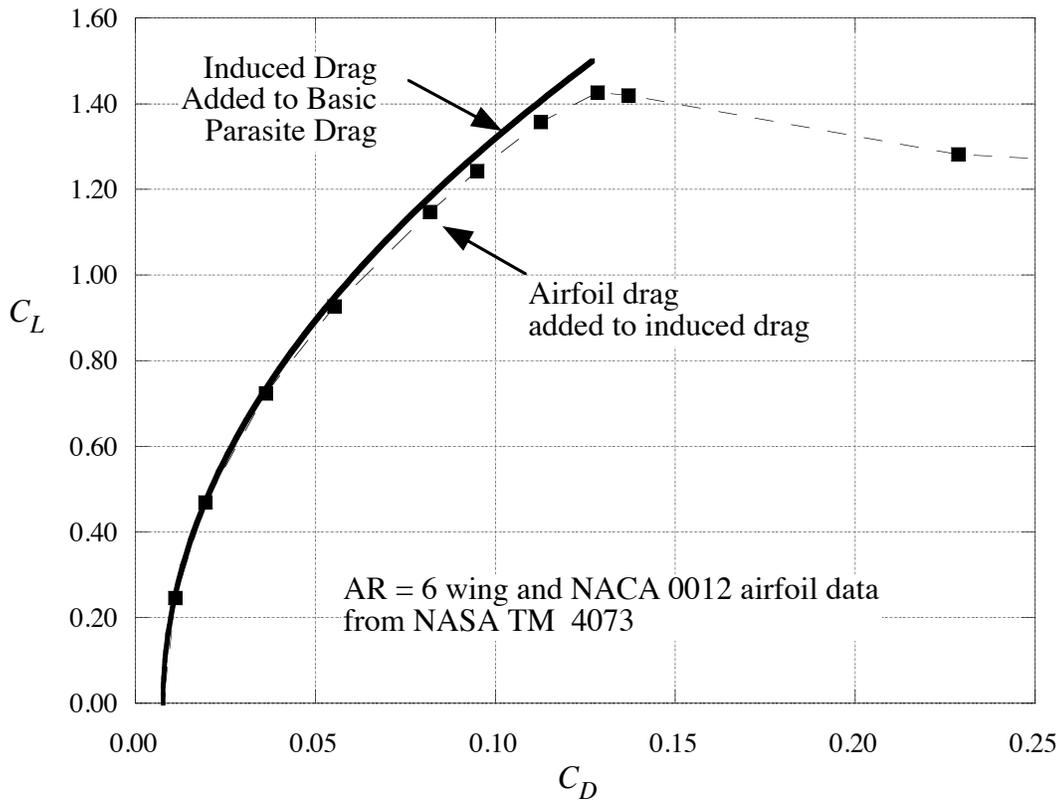
Figure 7. Drag polar for the  $AR = 6$  elliptical wing with NACA airfoil data, going all the way to  $C_{Lmax}$ . The airfoil drag is from NASA TM 4073, and the transition strip of 120 case was selected (as shown in Fig. 6).
