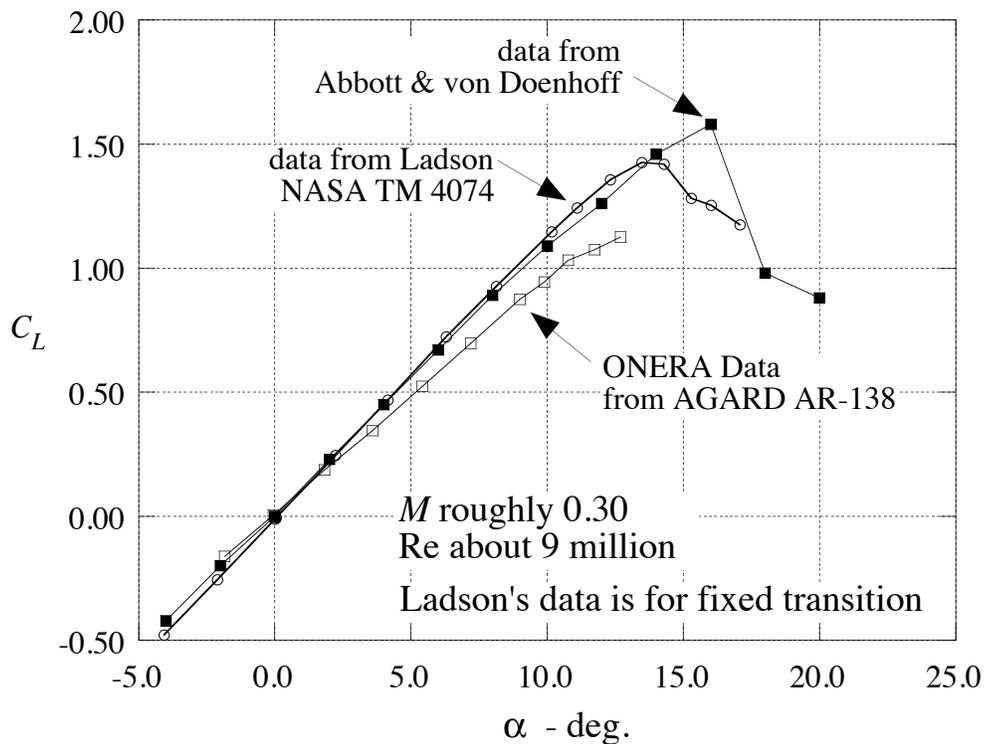
Figure 5. Comparison of three different sets of wind tunnel tests for the NACA 0012 airfoil at low speed.
