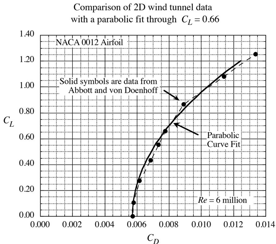
Figure 1. Comparison of NACA 0012 airfoil wing tunnel data with a parabolic curve fit.
