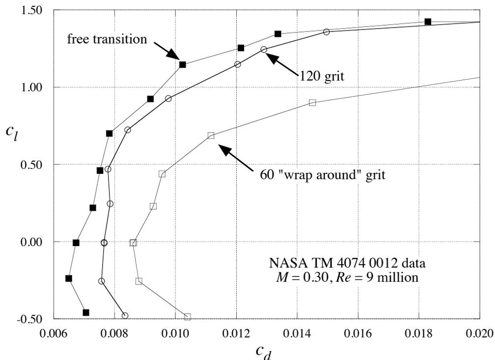
Figure 6. NASA TM 4074 WT Test of the NACA 0012 airfoil.
