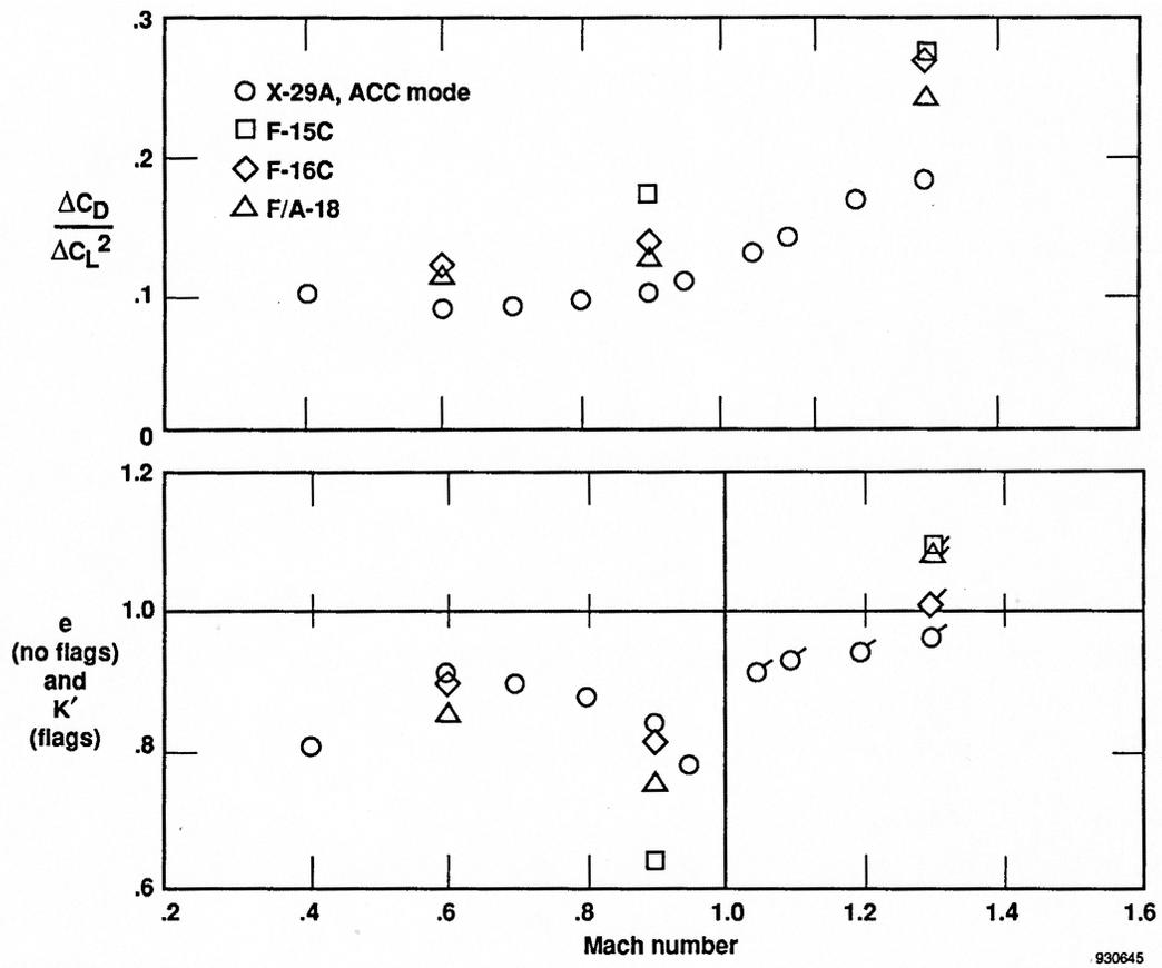
Figure 7. X-29 drag due to lift compared to other fighters (NASA TP 3414).
