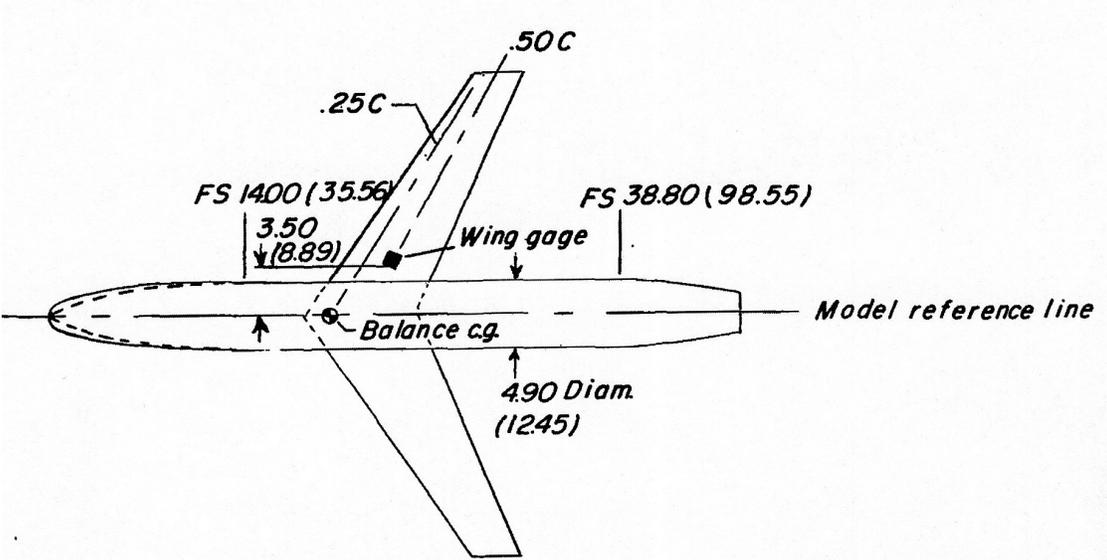
Figure 4. Wind Tunnel Model Planform (NASA TN D-5805)
