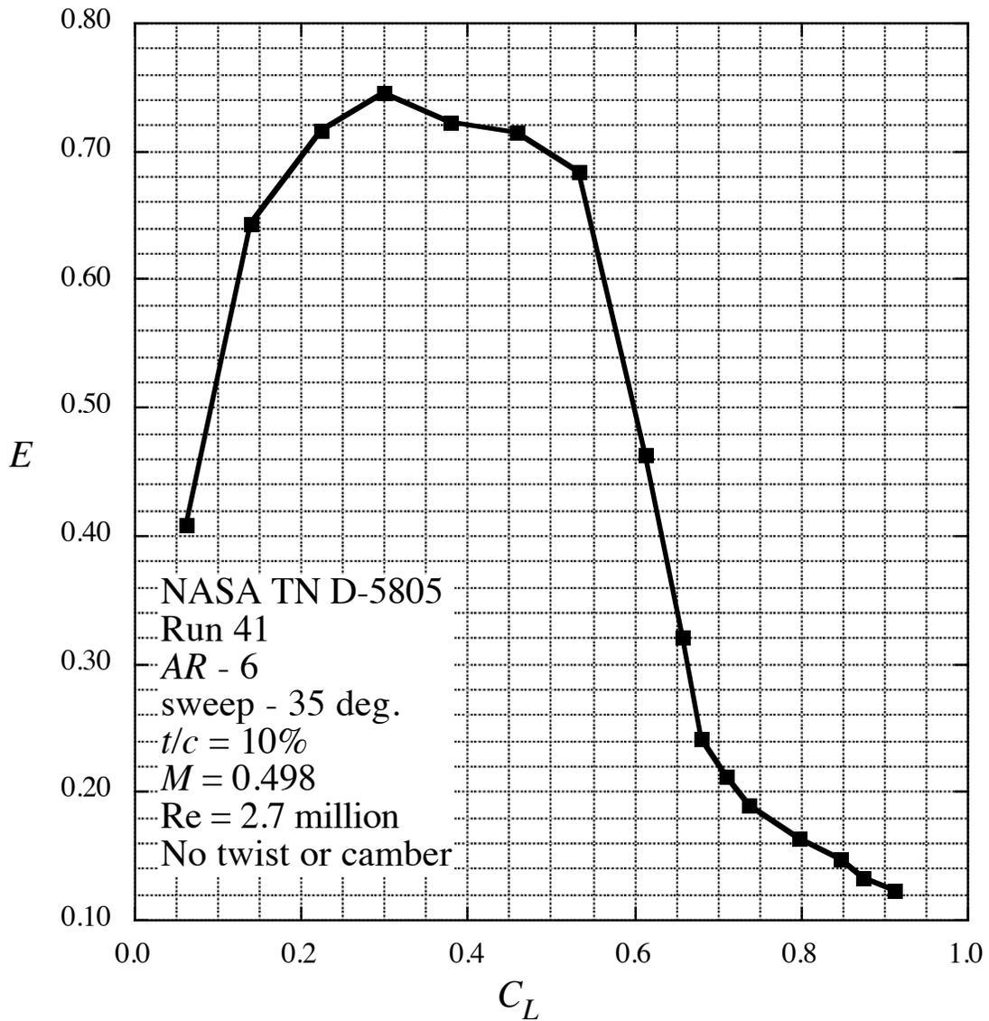
Figure 5.  $E$  extracted from wind tunnel test tab data(NASA TN D-5805)
