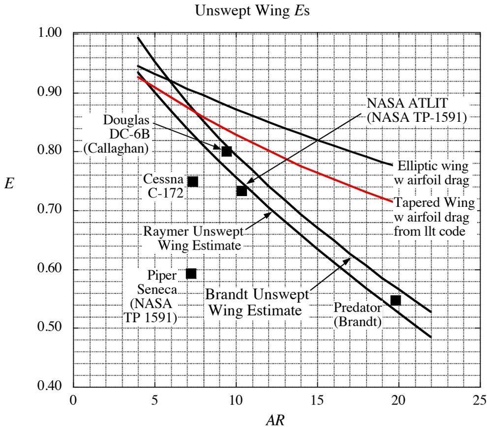
Figure 1. Brandt’s  $E$  estimate compared with Raymer’s Eqn 12.49 of the 4<sup>th</sup> Ed. and the value from the work in Curiosity 8 for an unswept wing and for a modified lifting line estimate.
