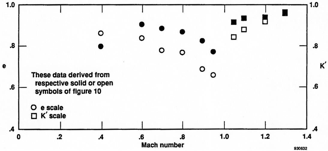
Figure 6. X-29 values of drag due to lift from NASA TP 3414 (solid symbols are from flight test)
