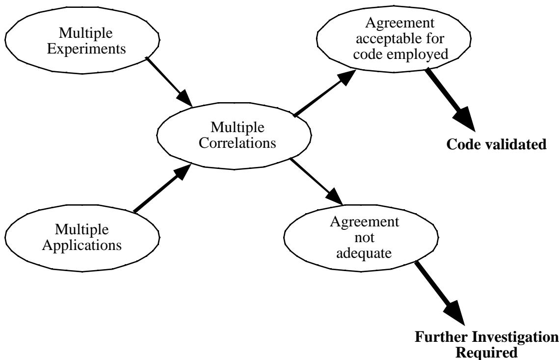
Figure 14-1. Required code development/validation steps needed before real application
