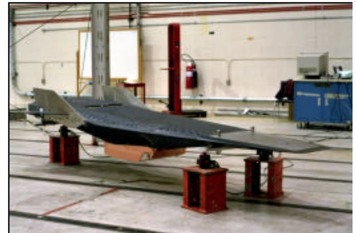
Ground Vibration Test
