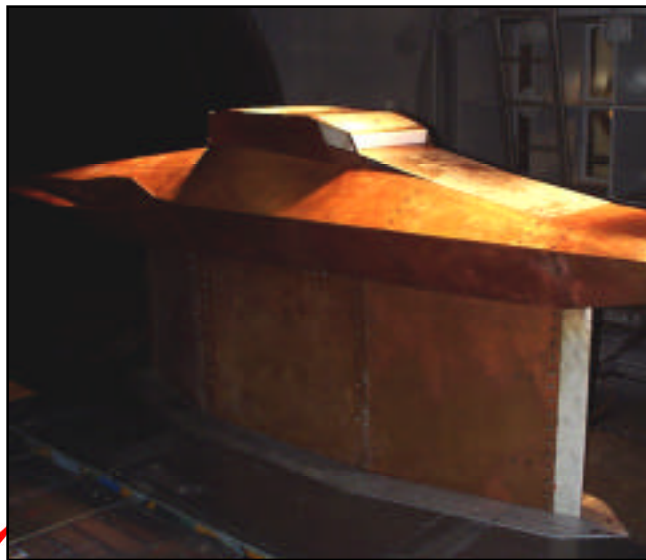
Engine in Langley 8-ft HTT
