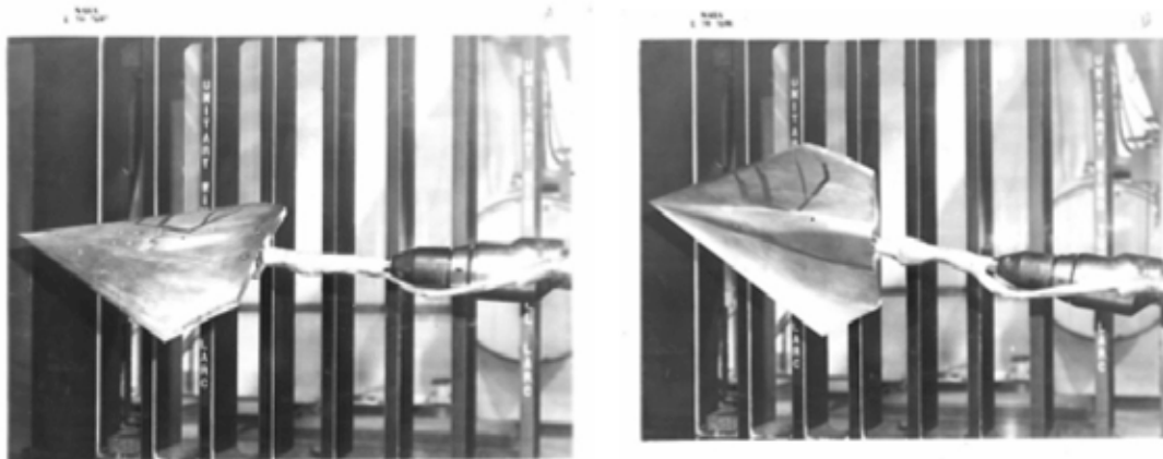
b) top and bottom views of the conceptual wing in the tunnel
