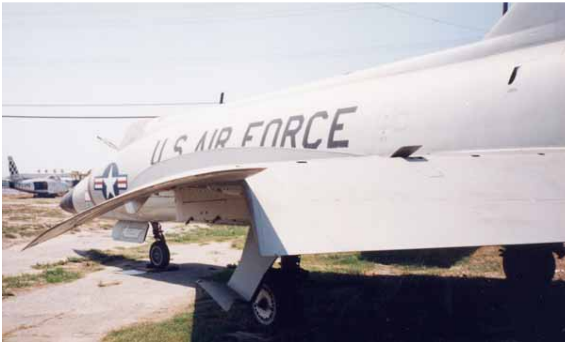
Figure 10-28. The F-102, showing the leading edge spanwise camber.
