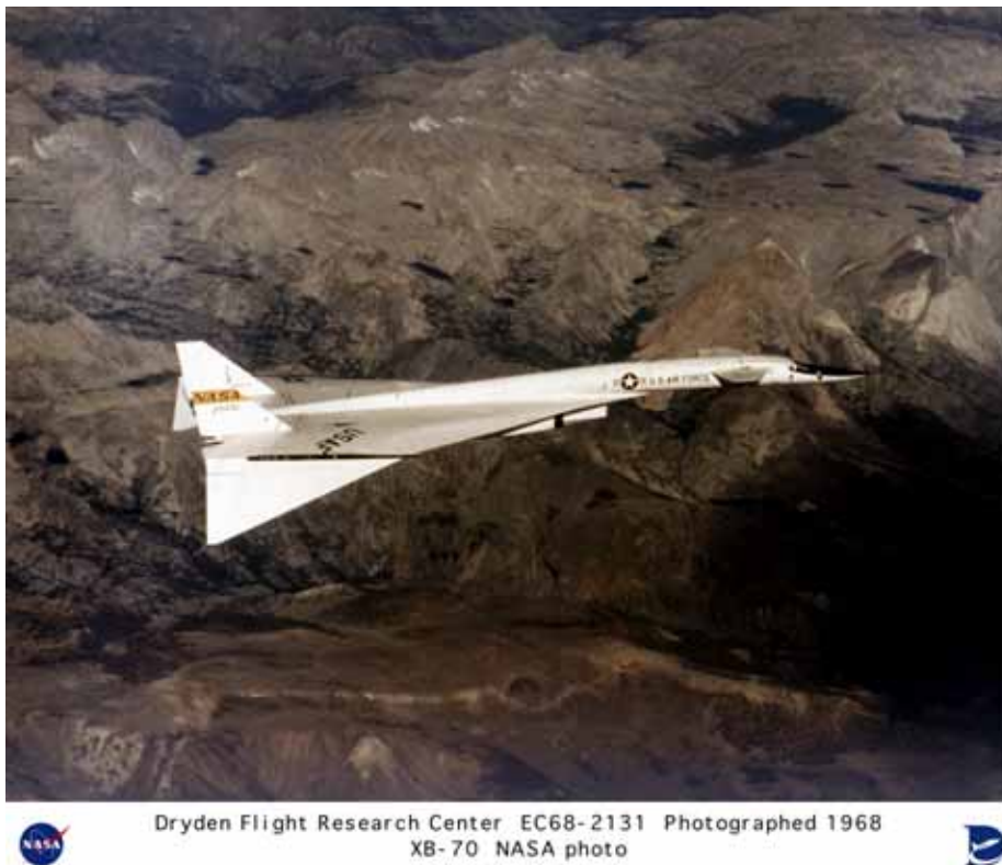
Figure 10-4. This figure shows the XB-70 flying with its wing tips deflected down.
