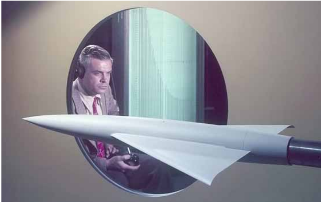
Figure 10-29. Conically cambered model in the NACA Ames Wind Tunnel (NASA Photo)
