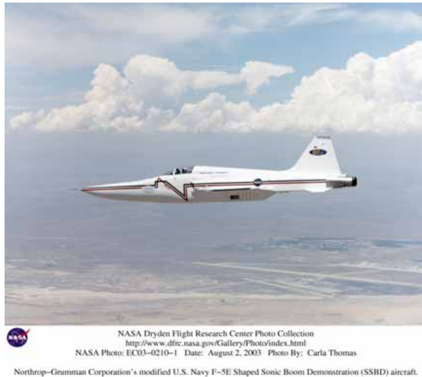
Figure 10-65 Demonstrator for the shaped boom test. (NASA Photo)
