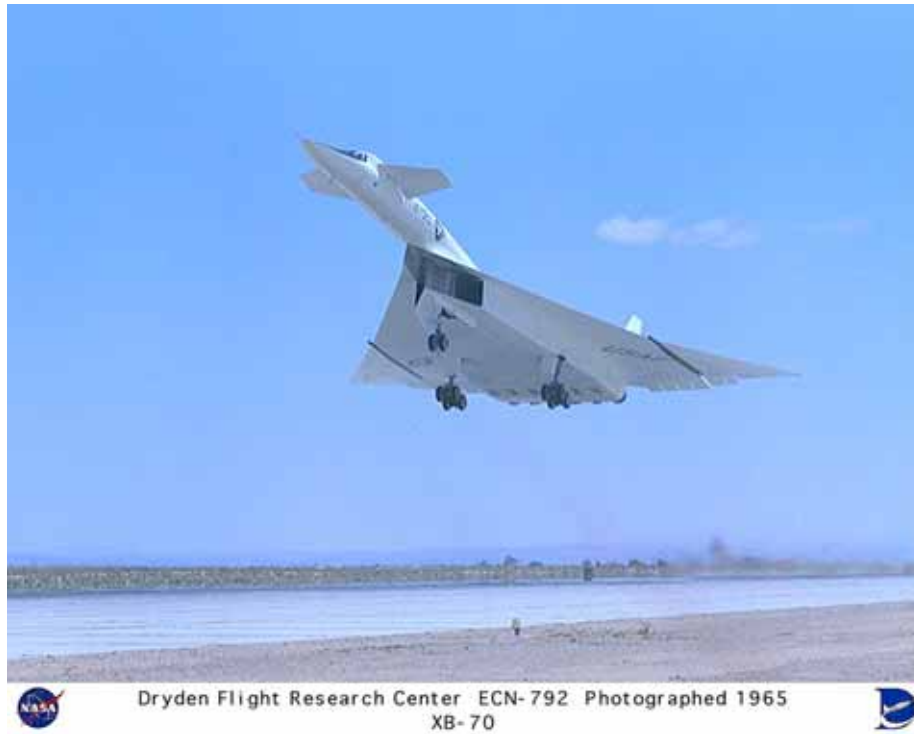
Figure 10-3. The XB-70 on takeoff. Note the large delta wing. The canard is essentially a trimmer.
