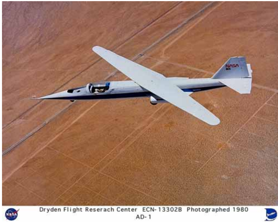
Figure 10-38. Oblique wing flight demonstration by the AD-1.
