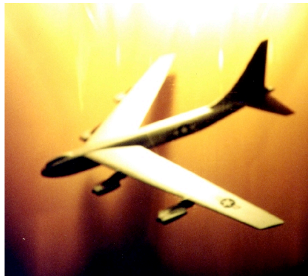
b) B-52 illustrating high-wing mount
