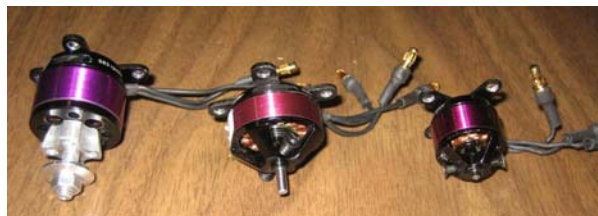
Figure 24 : From left to right: Hacker A20-30M, Hacker A20-24S, Hacker A10-9L
