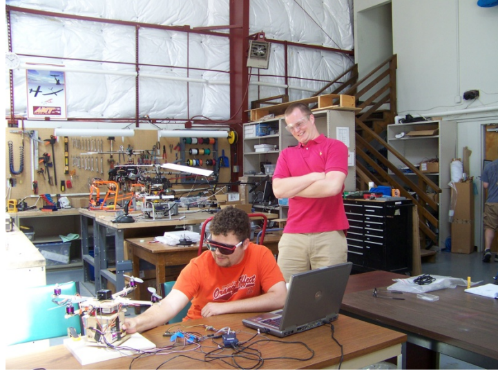
Figure 55: Yaw Controller Testing on Yaw Test Stand
