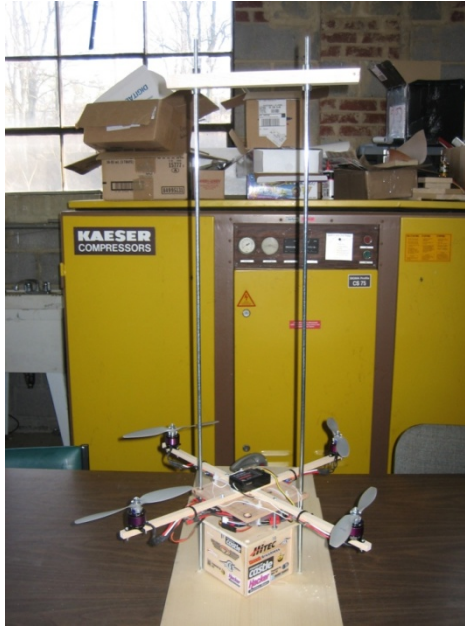
Figure 32 - The hover stand showing the two vertical rods attached to the wooden base.
