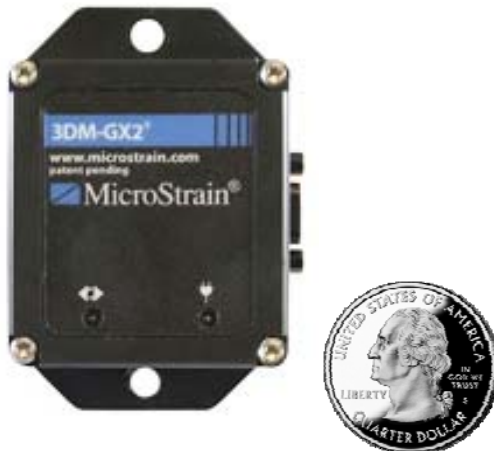
Figure 49: The Microstrain 3DM-GX2 IMU. [15]
