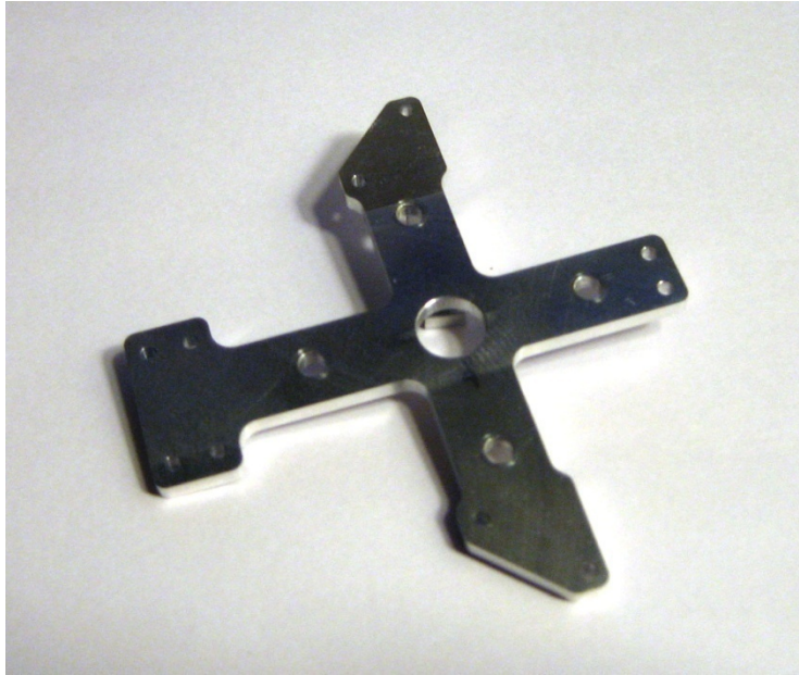
Figure 21: Motor mount base created on CNC machine.
