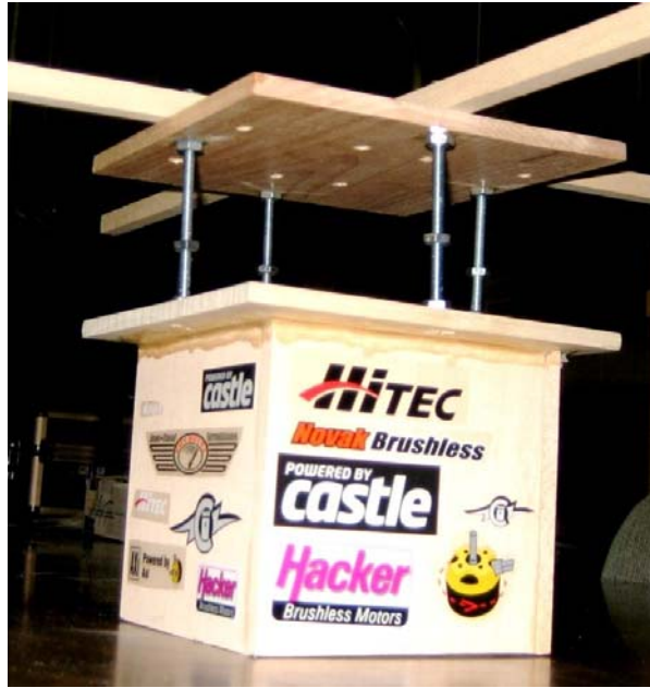
Figure 19: Bolts connecting base plate to ballast box
