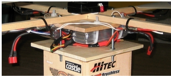
Figure 18: Batteries with open connections and other wires stored below the base plate
