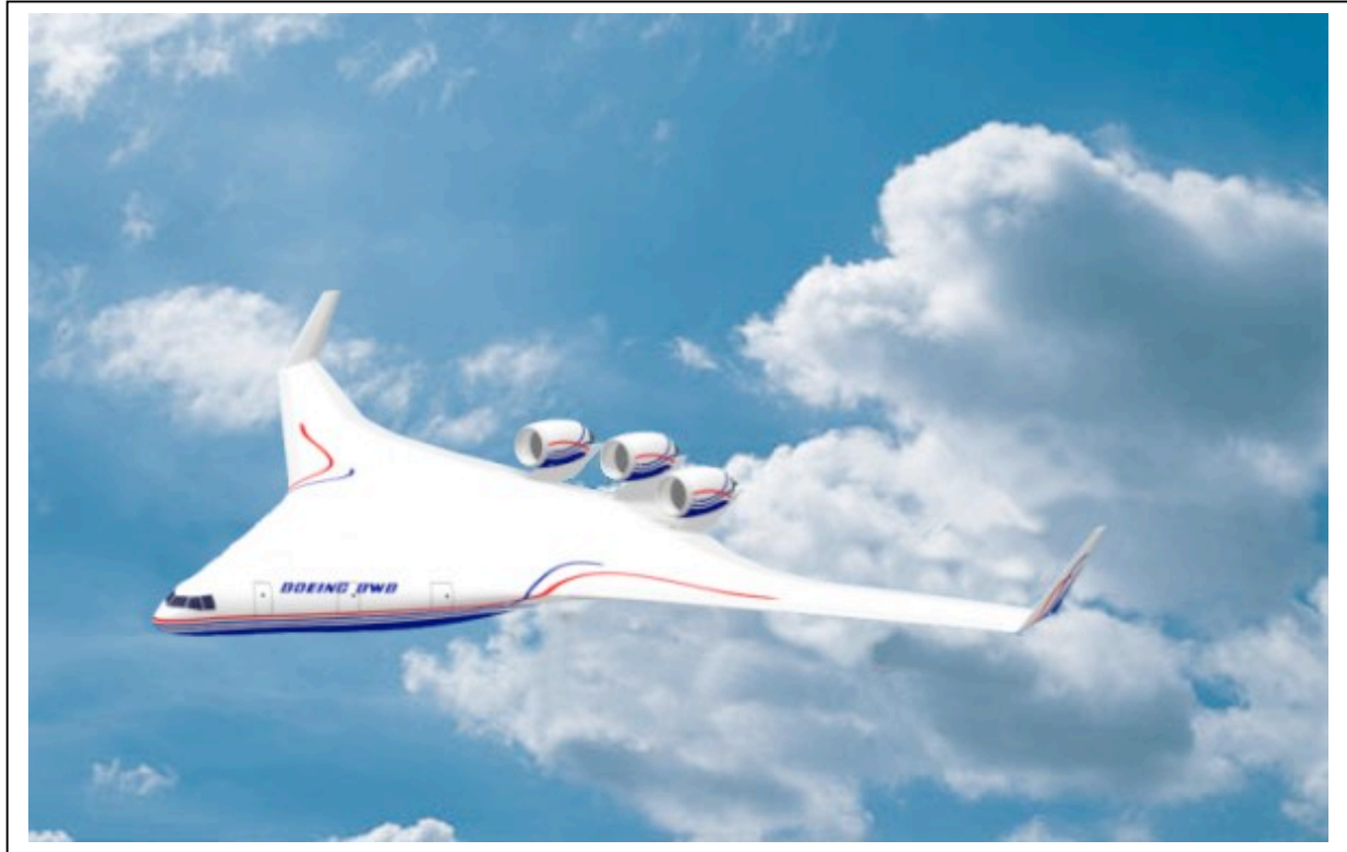
Figure 2. The Blended Wing Body Concept (courtesy Boeing)
