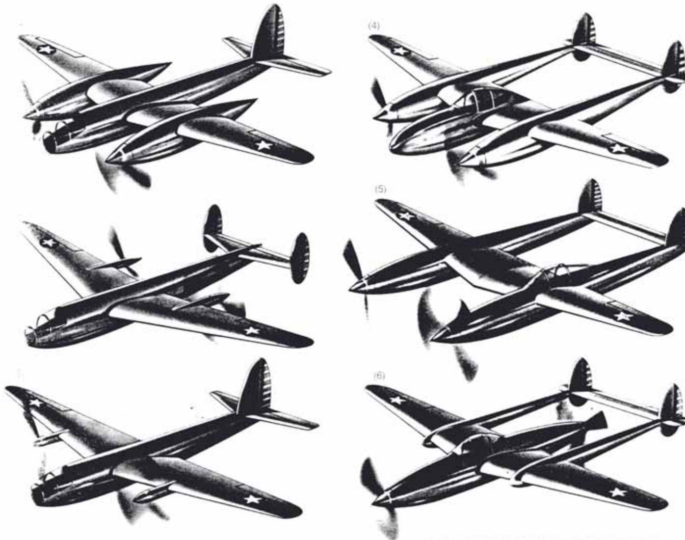
Kelly Johnson's six designs for 1937 Army fighter competition: (2) and (3) load two engines in each fuselage; (4) became XP-38.
