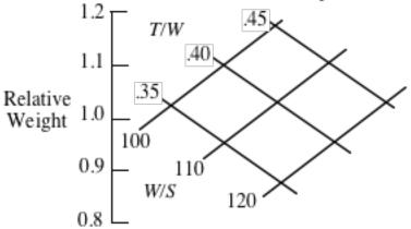
Step 2: shift scale, plot weights for various T/W, W/S held at constant 2
