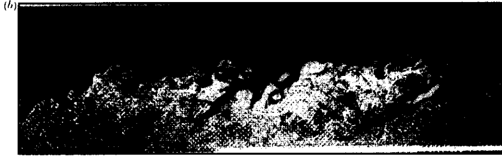
Figure 36: Flow visualization by Falco (1977), of a boundary layer at Re_\theta \approx 4,000 , obtained by seeding the flow with a fog of oil droplets, and illuminating the flow with a planar laser sheet. Flow is from left to right. Figure from Van Dyke (1982).
